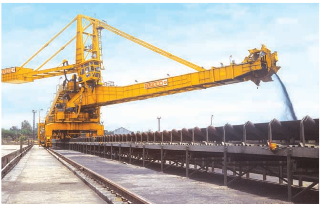
Stacker-Cum-Reclaimer in Operation at Thermal Power Station of Maharashtra State Electricity Board
